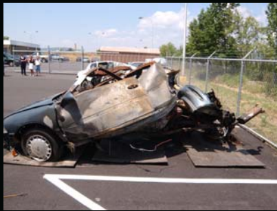
The impact may effect all possible alternative installation locations for the fuel tank.
