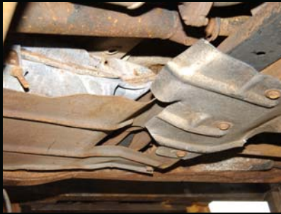
Often, components of the vehicle itself become the intruding objects into the fuel system.
